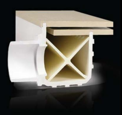
Zodiac's patented X-Baffle design allows water to rotate through chambers to ensure even flow when released from the nozzle. This technology ensures water is spread to all parts of water feature allowing it to hold its distinctive form for up to 1.2 metres.
